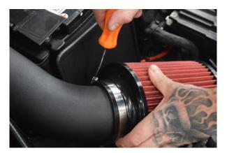
25. Tighten the Jubilee using a Flat Screwdriver, ensuring not to over tighten.
