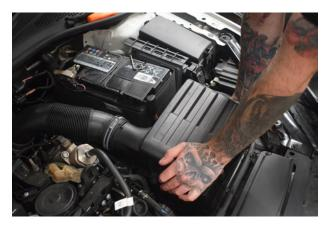
5. The OEM airbox can now be lifted from its mounting points.
