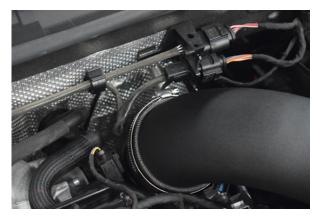
23. Tighten the jubilee clip on the throttle body inlet.
