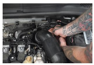
3. Undo jubilee clip on the OEM throttle body intake pipe.
