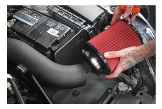
24. Place filter onto the opposite end of the hard pipe.
