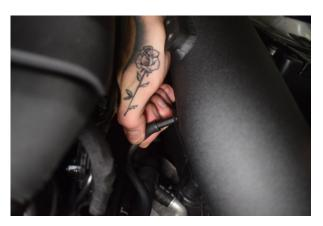
20. Install the breather pipe on to the new hard pipe.
