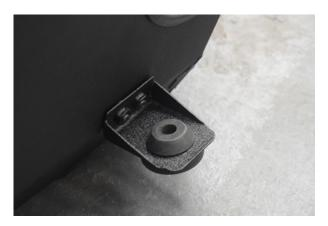
8. Install the bobbin into the bracket and install on the Direnza air box.
