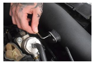
21. Once in position you can secure the support bracket to the hard pipe.
